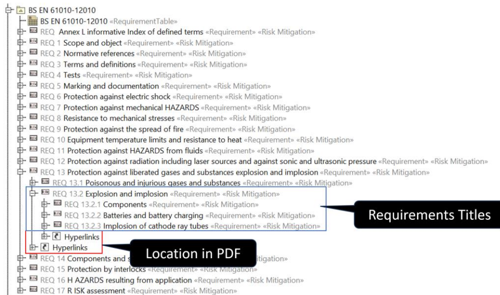
Figure 4 – A Snapshot for the SysML Norm Model for "BS EN 61010-12010"
